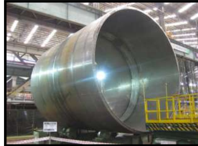
SG Upper Vessel - Unit 2A
